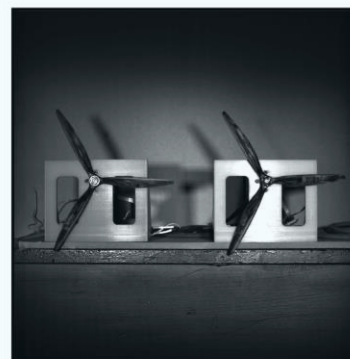
The high-speed camera view of the phased-locked propellers at \varphi=0^\circ
