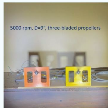
High-Speed camera setup for side-by-side configuration
