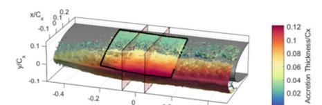
Full 3D Accretion measurements using OTI DIC imaging developments (taken in NRC AIWT facility).
