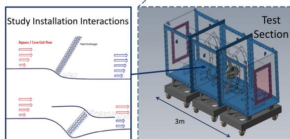
Tunnel Air Side, configured for turbofan bypass flow
