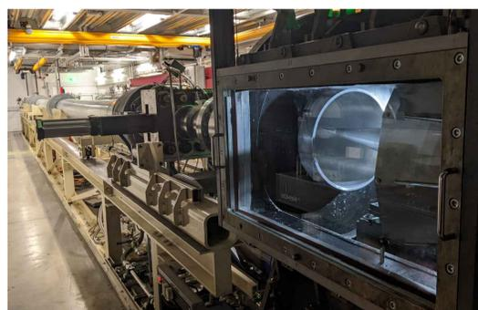
HDT ready to fire with a conical test article
